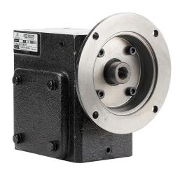
IronHorse heavy-duty worm gearbox, 60:1 ratio, NEMA 56C input, right hand, 1.125in diameter output shaft, nominal 0.86hp at 1.0 SF, 1149 lb-in mechanical output torque, 2-3/8in center distance, cast iron housing, tapped-base mount.
