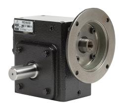
IronHorse heavy-duty worm gearbox, 60:1 ratio, 56C-Face input, left hand, 1.125in diameter output shaft, nominal 0.5hp at 1.0 SF, 1149 lb-in mechanical output torque, 2-3/8in center distance, cast iron housing, tapped-base mount.
