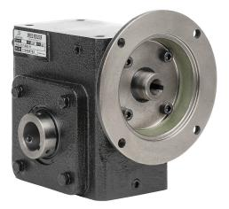
IronHorse heavy-duty worm gearbox, 60:1 ratio, 56C-Face input, hollow, 1.25in diameter output shaft, nominal 0.5hp at 1.0 SF, 1149 lb-in mechanical output torque, 2-3/8in center distance, cast iron housing, tapped-base mount.
