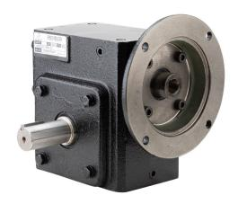
IronHorse heavy-duty worm gearbox, 60:1 ratio, 56C-Face input, dual, 1.125in diameter output shaft, nominal 0.5hp at 1.0 SF, 1149 lb-in mechanical output torque, 2-3/8in center distance, cast iron housing, tapped-base mount.
