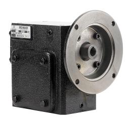
IronHorse heavy-duty worm gearbox, 40:1 ratio, 56C-Face input, right hand, 1.125in diameter output shaft, nominal 0.5hp at 1.0 SF, 1483 lb-in mechanical output torque, 2-3/8in center distance, cast iron housing, tapped-base mount.
