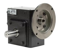
IronHorse heavy-duty worm gearbox, 40:1 ratio, 56C-Face input, left hand, 1.125in diameter output shaft, nominal 0.5hp at 1.0 SF, 1483 lb-in mechanical output torque, 2-3/8in center distance, cast iron housing, tapped-base mount.
