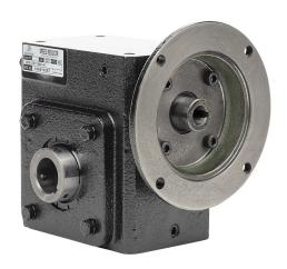
IronHorse heavy-duty worm gearbox, 40:1 ratio, 56C-Face input, hollow, 1.25in diameter output shaft, nominal 0.5hp at 1.0 SF, 1483 lb-in mechanical output torque, 2-3/8in center distance, cast iron housing, tapped-base mount.
