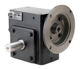
IronHorse heavy-duty worm gearbox, 40:1 ratio, 56C-Face input, dual, 1.125in diameter output shaft, nominal 0.5hp at 1.0 SF, 1483 lb-in mechanical output torque, 2-3/8in center distance, cast iron housing, tapped-base mount.
