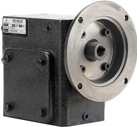
IronHorse heavy-duty worm gearbox, 20:1 ratio, 56C-Face input, right hand, 1.125in diameter output shaft, nominal 1hp at 1.0 SF, 1195 lb-in mechanical output torque, 2-3/8in center distance, cast iron housing, tapped-base mount.
