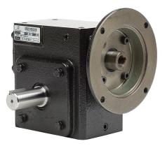
IronHorse heavy-duty worm gearbox, 20:1 ratio, 56C-Face input, left hand, 1.125in diameter output shaft, nominal 1hp at 1.0 SF, 1195 lb-in mechanical output torque, 2-3/8in center distance, cast iron housing, tapped-base mount.
