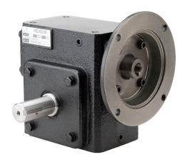
IronHorse heavy-duty worm gearbox, 20:1 ratio, 56C-Face input, dual, 1.125in diameter output shaft, nominal 1hp at 1.0 SF, 1195 lb-in mechanical output torque, 2-3/8in center distance, cast iron housing, tapped-base mount.
