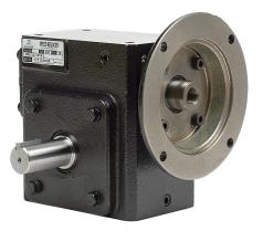
IronHorse heavy-duty worm gearbox, 15:1 ratio, 56C-Face input, left hand, 1.125in diameter output shaft, nominal 1hp at 1.0 SF, 1249 lb-in mechanical output torque, 2-3/8in center distance, cast iron housing, tapped-base mount.
