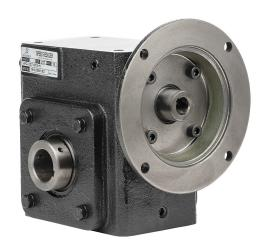
IronHorse heavy-duty worm gearbox, 15:1 ratio, 56C-Face input, hollow, 1.25in diameter output shaft, nominal 1hp at 1.0 SF, 1249 lb-in mechanical output torque, 2-3/8in center distance, cast iron housing, tapped-base mount.
