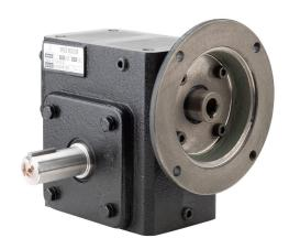
IronHorse heavy-duty worm gearbox, 15:1 ratio, 56C-Face input, dual, 1.125in diameter output shaft, nominal 1hp at 1.0 SF, 1249 lb-in mechanical output torque, 2-3/8in center distance, cast iron housing, tapped-base mount.
