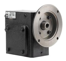
IronHorse heavy-duty worm gearbox, 10:1 ratio, 56C-Face input, right hand, 1.125in diameter output shaft, nominal 1.5hp at 1.0 SF, 1158 lb-in mechanical output torque, 2-3/8in center distance, cast iron housing, tapped-base mount.
