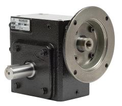
IronHorse heavy-duty worm gearbox, 10:1 ratio, 56C-Face input, left hand, 1.125in diameter output shaft, nominal 1.5hp at 1.0 SF, 1158 lb-in mechanical output torque, 2-3/8in center distance, cast iron housing, tapped-base mount.
