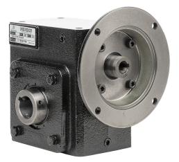
IronHorse heavy-duty worm gearbox, 10:1 ratio, 56C-Face input, hollow, 1.25in diameter output shaft, nominal 1.5hp at 1.0 SF, 1158 lb-in mechanical output torque, 2-3/8in center distance, cast iron housing, tapped-base mount.
