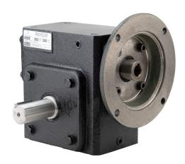
IronHorse heavy-duty worm gearbox, 10:1 ratio, 56C-Face input, dual, 1.125in diameter output shaft, nominal 1.5hp at 1.0 SF, 1158 lb-in mechanical output torque, 2-3/8in center distance, cast iron housing, tapped-base mount.
