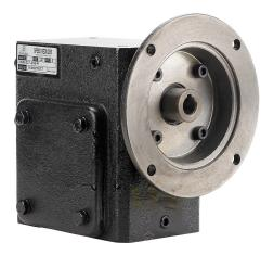
IronHorse heavy-duty worm gearbox, 5:1 ratio, 56C-Face input, right hand, 1.125in diameter output shaft, nominal 3hp at 1.0 SF, 766 lb-in mechanical output torque, 2-3/8in center distance, cast iron housing, tapped-base mount.
