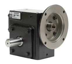
IronHorse heavy-duty worm gearbox, 5:1 ratio, 56C-Face input, left hand, 1.125in diameter output shaft, nominal 3hp at 1.0 SF, 766 lb-in mechanical output torque, 2-3/8in center distance, cast iron housing, tapped-base mount.
