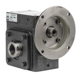
IronHorse heavy-duty worm gearbox, 5:1 ratio, 56C-Face input, hollow, 1.25in diameter output shaft, nominal 3hp at 1.0 SF, 766 lb-in mechanical output torque, 2-3/8in center distance, cast iron housing, tapped-base mount.
