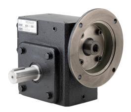
IronHorse heavy-duty worm gearbox, 5:1 ratio, 56C-Face input, dual, 1.125in diameter output shaft, nominal 3hp at 1.0 SF, 766 lb-in mechanical output torque, 2-3/8in center distance, cast iron housing, tapped-base mount.
