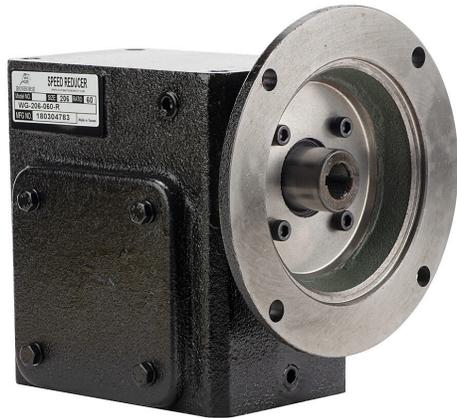
IronHorse heavy-duty worm gearbox, 60:1 ratio, 56C-Face input, right hand, 1in diameter output shaft, nominal 0.33hp at 1.0 SF, 750 lb-in mechanical output torque, 2-1/16in center distance, cast iron housing, tapped-base mount.
