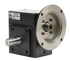
IronHorse heavy-duty worm gearbox, 60:1 ratio, 56C-Face input, left hand, 1in diameter output shaft, nominal 0.33hp at 1.0 SF, 750 lb-in mechanical output torque, 2-1/16in center distance, cast iron housing, tapped-base mount.
