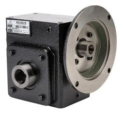
IronHorse heavy-duty worm gearbox, 60:1 ratio, 56C-Face input, hollow, 1.125in diameter output shaft, nominal 0.33hp at 1.0 SF, 750 lb-in mechanical output torque, 2-1/16in center distance, cast iron housing, tapped-base mount.
