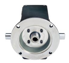
IronHorse heavy-duty worm gearbox, 60:1 ratio, 56C-Face input, dual, 1in diameter output shaft, nominal 0.33hp at 1.0 SF, 750 lb-in mechanical output torque, 2-1/16in center distance, cast iron housing, tapped-base mount.
