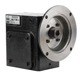
IronHorse heavy-duty worm gearbox, 40:1 ratio, 56C-Face input, right hand, 1in diameter output shaft, nominal 0.5hp at 1.0 SF, 1120 lb-in mechanical output torque, 2-1/16in center distance, cast iron housing, tapped-base mount.
