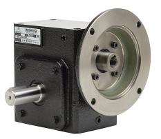
IronHorse heavy-duty worm gearbox, 40:1 ratio, 56C-Face input, left hand, 1in diameter output shaft, nominal 0.5hp at 1.0 SF, 1120 lb-in mechanical output torque, 2-1/16in center distance, cast iron housing, tapped-base mount.
