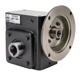
IronHorse heavy-duty worm gearbox, 40:1 ratio, 56C-Face input, hollow, 1.125in diameter output shaft, nominal 0.5hp at 1.0 SF, 1120 lb-in mechanical output torque, 2-1/16in center distance, cast iron housing, tapped-base mount.
