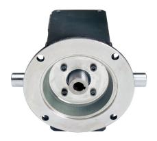
IronHorse heavy-duty worm gearbox, 40:1 ratio, 56C-Face input, dual, 1in diameter output shaft, nominal 0.5hp at 1.0 SF, 1120 lbin mechanical output torque, 2-1/16in center distance, cast iron housing, tapped-base mount.
