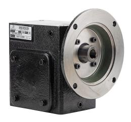
IronHorse heavy-duty worm gearbox, 20:1 ratio, 56C-Face input, right hand, 1in diameter output shaft, nominal 1hp at 1.0 SF, 914 lb-in mechanical output torque, 2-1/16in center distance, cast iron housing, tapped-base mount.
