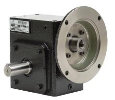
IronHorse heavy-duty worm gearbox, 20:1 ratio, 56C-Face input, left hand, 1in diameter output shaft, nominal 1hp at 1.0 SF, 914 lbin mechanical output torque, 2-1/16in center distance, cast iron housing, tapped-base mount.
