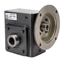
IronHorse heavy-duty worm gearbox, 20:1 ratio, 56C-Face input, hollow, 1.125in diameter output shaft, nominal 1hp at 1.0 SF, 914 lb-in mechanical output torque, 2-1/16in center distance, cast iron housing, tapped-base mount.
