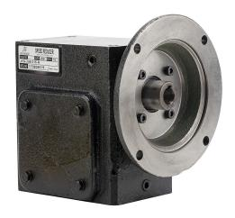
IronHorse heavy-duty worm gearbox, 15:1 ratio, 56C-Face input, right hand, 1in diameter output shaft, nominal 1hp at 1.0 SF, 1002 lb-in mechanical output torque, 2-1/16in center distance, cast iron housing, tapped-base mount.
