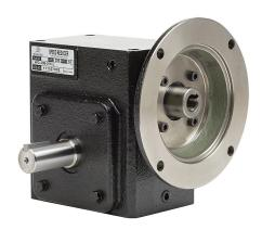
IronHorse heavy-duty worm gearbox, 15:1 ratio, 56C-Face input, left hand, 1in diameter output shaft, nominal 1hp at 1.0 SF, 1002 lb-in mechanical output torque, 2-1/16in center distance, cast iron housing, tapped-base mount.
