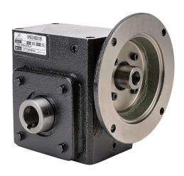
IronHorse heavy-duty worm gearbox, 15:1 ratio, 56C-Face input, hollow, 1.125in diameter output shaft, nominal 1hp at 1.0 SF, 1002 lb-in mechanical output torque, 2-1/16in center distance, cast iron housing, tapped-base mount.
