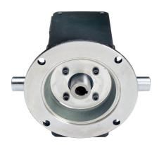
IronHorse heavy-duty worm gearbox, 15:1 ratio, 56C-Face input, dual, 1in diameter output shaft, nominal 1hp at 1.0 SF, 1002 lb-in mechanical output torque, 2-1/16in center distance, cast iron housing, tapped-base mount.
