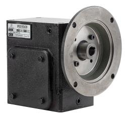
IronHorse heavy-duty worm gearbox, 10:1 ratio, 56C-Face input, right hand, 1in diameter output shaft, nominal 1.5hp at 1.0 SF, 935 lb-in mechanical output torque, 2-1/16in center distance, cast iron housing, tapped-base mount.
