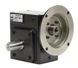
IronHorse heavy-duty worm gearbox, 10:1 ratio, 56C-Face input, left hand, 1in diameter output shaft, nominal 1.5hp at 1.0 SF, 935 lb-in mechanical output torque, 2-1/16in center distance, cast iron housing, tapped-base mount.
