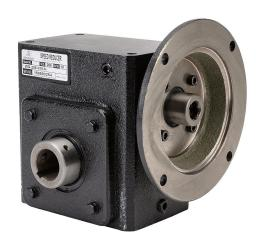
IronHorse heavy-duty worm gearbox, 10:1 ratio, 56C-Face input, hollow, 1.125in diameter output shaft, nominal 1.5hp at 1.0 SF, 935 lb-in mechanical output torque, 2-1/16in center distance, cast iron housing, tapped-base mount.
