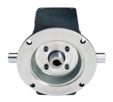
IronHorse heavy-duty worm gearbox, 10:1 ratio, 56C-Face input, dual, 1in diameter output shaft, nominal 1.5hp at 1.0 SF, 935 lb-in mechanical output torque, 2-1/16in center distance, cast iron housing, tapped-base mount.
