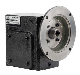
IronHorse heavy-duty worm gearbox, 5:1 ratio, 56C-Face input, right hand, 1in diameter output shaft, nominal 2hp at 1.0 SF, 925 lb-in mechanical output torque, 2-1/16in center distance, cast iron housing, tapped-base mount.
