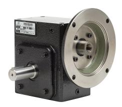
IronHorse heavy-duty worm gearbox, 5:1 ratio, 56C-Face input, left hand, 1in diameter output shaft, nominal 2hp at 1.0 SF, 925 lb-in mechanical output torque, 2-1/16in center distance, cast iron housing, tapped-base mount.
