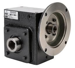
IronHorse heavy-duty worm gearbox, 5:1 ratio, 56C-Face input, hollow, 1.125in diameter output shaft, nominal 2hp at 1.0 SF, 925 Ib-in mechanical output torque, 2-1/16in center distance, cast iron housing, tapped-base mount.
