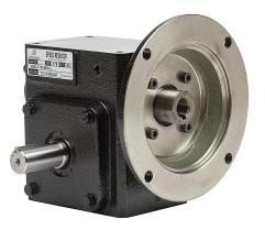
IronHorse heavy-duty worm gearbox, 60:1 ratio, 56C-Face input, left hand, 0.875in diameter output shaft, nominal 0.25hp at 1.0 SF, 433 lb-in mechanical output torque, 1-3/4in center distance, cast iron housing, tapped-base mount.
