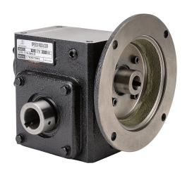
IronHorse heavy-duty worm gearbox, 60:1 ratio, 56C-Face input, hollow, 1in diameter output shaft, nominal 0.25hp at 1.0 SF, 433 lb-in mechanical output torque, 1-3/4in center distance, cast iron housing, tapped-base mount.
