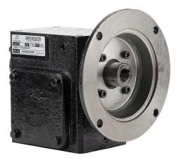
IronHorse heavy-duty worm gearbox, 40:1 ratio, 56C-Face input, right hand, 0.875in diameter output shaft, nominal 0.33hp at 1.0 SF, 714 lb-in mechanical output torque, 1-3/4in center distance, cast iron housing, tapped-base mount.
