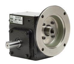
IronHorse heavy-duty worm gearbox, 40:1 ratio, 56C-Face input, left hand, 0.875in diameter output shaft, nominal 0.33hp at 1.0 SF, 714 lb-in mechanical output torque, 1-3/4in center distance, cast iron housing, tapped-base mount.
