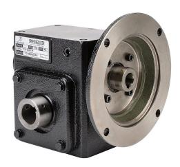
IronHorse heavy-duty worm gearbox, 40:1 ratio, 56C-Face input, hollow, 1in diameter output shaft, nominal 0.33hp at 1.0 SF, 714 lb-in mechanical output torque, 1-3/4in center distance, cast iron housing, tapped-base mount.
