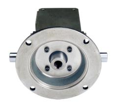
IronHorse heavy-duty worm gearbox, 40:1 ratio, 56C-Face input, dual, 0.875in diameter output shaft, nominal 0.33hp at 1.0 SF, 714 lb-in mechanical output torque, 1-3/4in center distance, cast iron housing, tapped-base mount.
